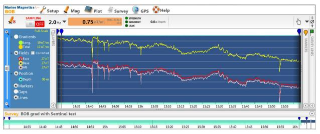
Figure 6-12 - Base station data (yellow trace) looks very similar to the towed magnetometer data (red and pink traces)
