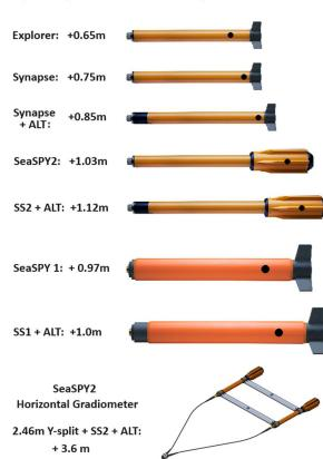
Layback adjustment for different magnetometer models
