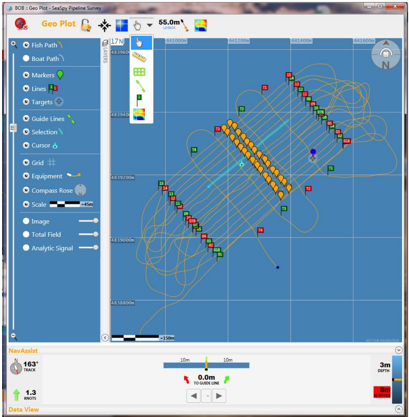
Figure 2 - BOB GeoPlot window with Layers panel, a drop-down tool bar, and the NavAssist panel The cyan selection and cursor show survey line 8, currently displayed on the MagPlot. The orange markers show pipeline anomalies on each line, while the blue marker shows another anomaly, an anchor, and its associated target mark. (The Targets feature is only available as part of the BOB Analysis Module extension) The NavAssist panel uses a guide line grid (if one was set up) for navigation assistance.
