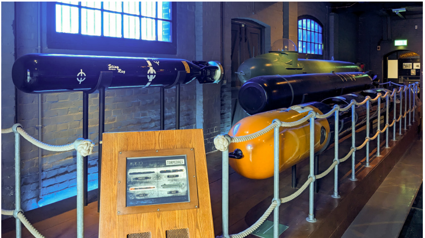
Display of free from explosive torpedoes of the Explosion Museum of Naval Firepower, Portsmouth, UK. In black with white markings, the lightweight Sting Ray (45 kg of high explosive, shaped charge, 1983), and the heavyweight Mark 24 Tigerfish (134 kg of high explosive, 1983), of the UK Royal Navy. In the bottom right the US Navy Mark 11 (227 kg of high explosive, 1926). In the back, the Neger, a Second World War German torpedo carrying craft. © The wub
