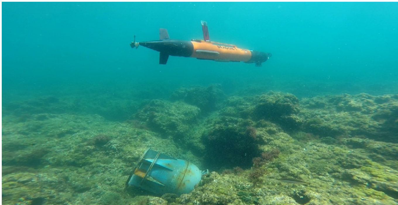
A light autonomous underwater vehicle scanning the sea bottom. These systems can efficiently deploy a wide range of survey sensors, reducing the logistical burden and risks associated to deploying EOD divers. © Portuguese Navy
