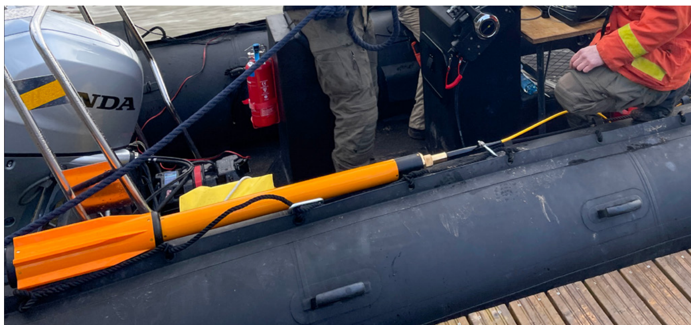
Towed magnetometer deployed in a small vessel. One of the challenges of deploying these systems is that they are much more difficult to adapt to variations in the seabed profile. Autonomous underwater vehicles which can automatically adjust distance to the seabed profile are becoming therefore more and more used, when depths allow its use. © Marine Magnetics
