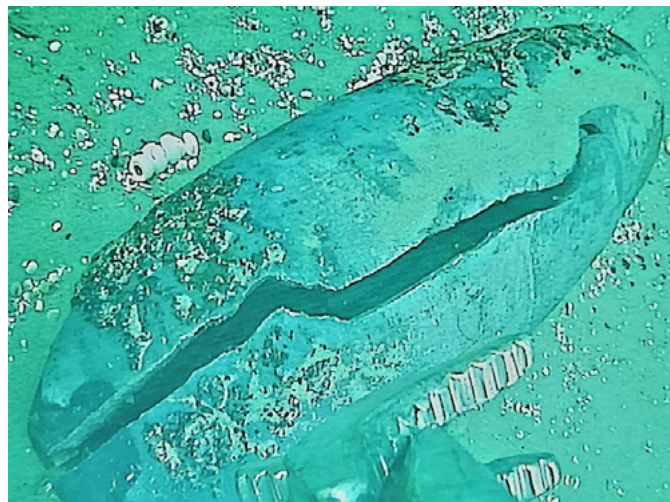
On the left, an underwater shaped charge positioned to dispose of an unexploded ordnance (air dropped bomb) by low order deflagration. On the right, the result of a successful deflagration underwater. This disposal method mitigates impact on marine life and underwater structures. © Helix Robotic Solutions Ltd
