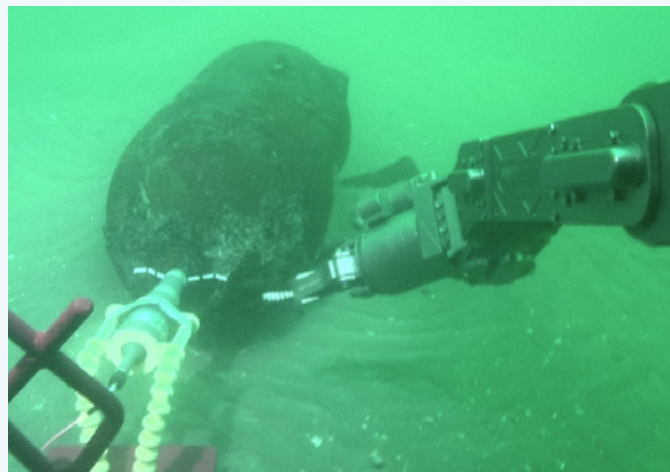
On the left, a remotely operated vehicle digging up an unexploded ordnance (air dropped bomb). On the right, the robotic arm of the remotely operated vehicle helps the placement of a low order deflagration shaped charge. © Helix Robotic Solutions Ltd
