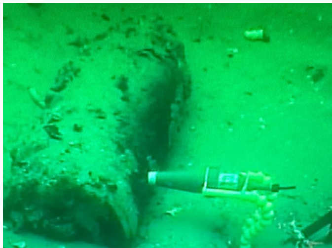
On the left, an underwater shaped charge positioned to dispose of an unexploded ordnance (air dropped bomb) by low order deflagration. On the right, the result of a successful deflagration underwater. This disposal method mitigates impact on marine life and underwater structures. © Helix Robotic Solutions Ltd
