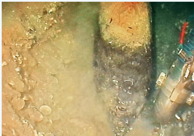
On the left, a remotely operated vehicle digging up an unexploded ordnance (air dropped bomb). On the right, the robotic arm of the remotely operated vehicle helps the placement of a low order deflagration shaped charge. © Helix Robotic Solutions Ltd
