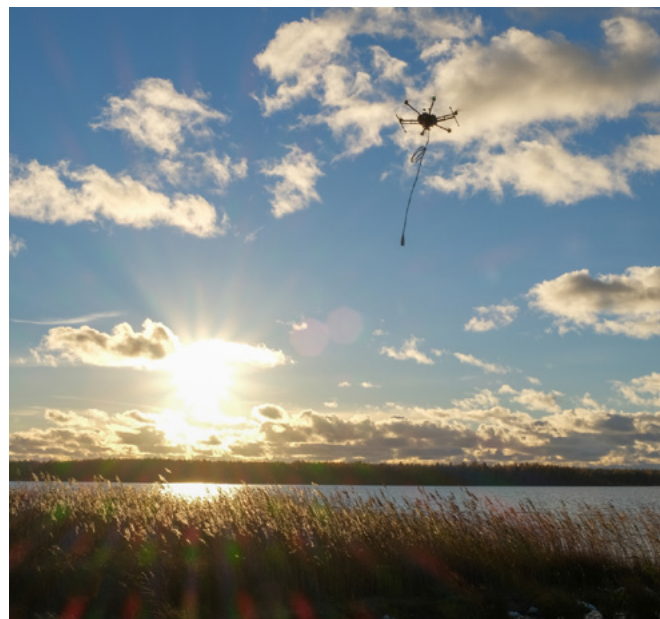
Towed magnetometer deployed in an uncrewed aerial vehicle. The use of water surface magnetometer survey is particularly efficient in shallow waters, including coastal transition areas, where vessels towed systems can't be used to systematically survey. © Marine Magnetics
