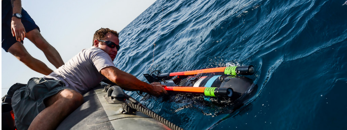
EOD operator retrieves the remotely operated vehicle Seafox during exercise. This is an expendable sea mine disposal vehicle. © U.S. Naval Forces Central Command/U.S. Fifth Fleet
