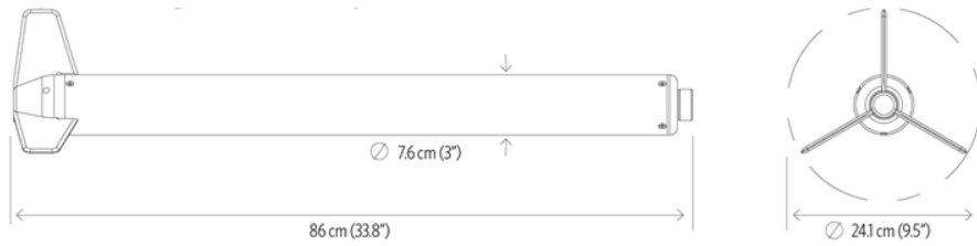
Figure 9-2 -Current 1000m Explorer towfish dimensions (3" orange tube). Manufactured after 2020.
