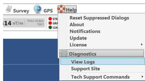
There may be rare situations where the magnetometer will continue taking readings and sending data to the COM port even if sampling accidentally gets turned OFF. Although these readings will not be saved into the survey database, they may still get saved into diagnostic logs, from which data may be subsequently recovered in an emergency.
