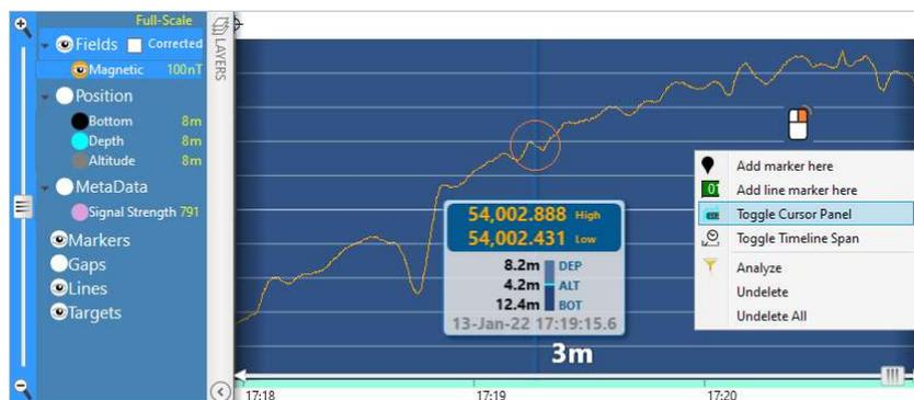
Figure 4-8: Profile Plot cursor panel shows readings at the cursor position
