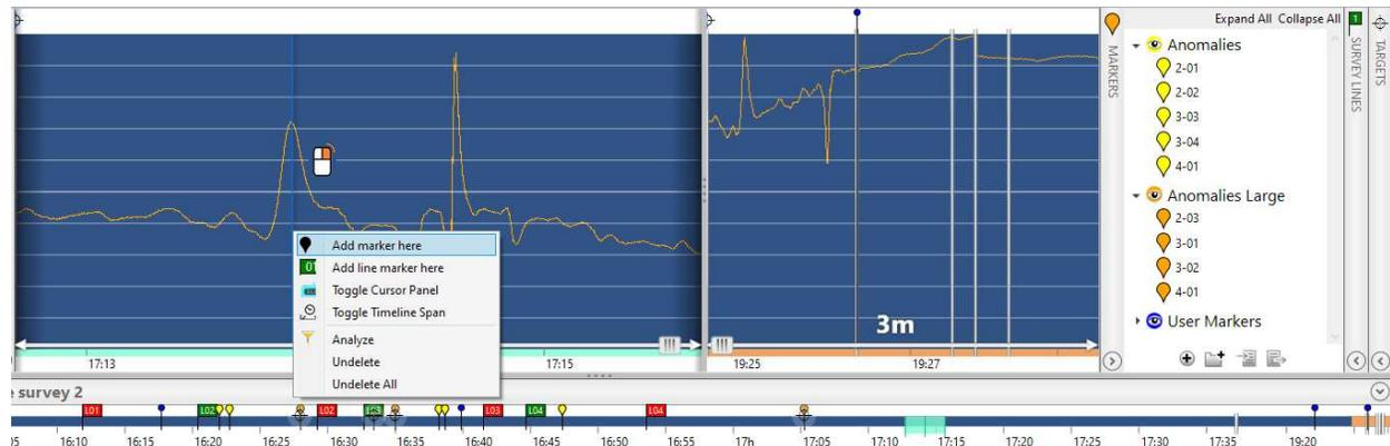
Figure 4-10: To add a marker to the profile, right click on the specific point and select “Add marker here”. Assigning colors to marker sets helps distinguish them on the timeline, profile and map view.
