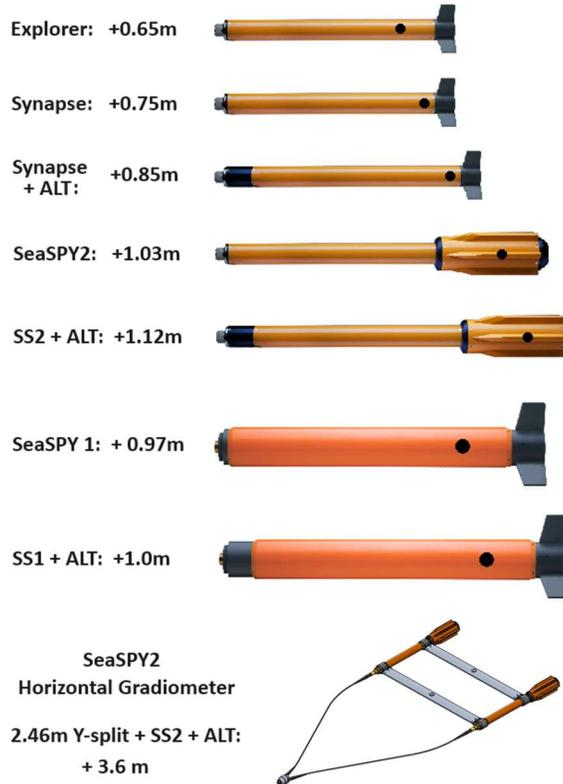
Figure 3-7: Towfish length needs to be accounted for when determining the layback
