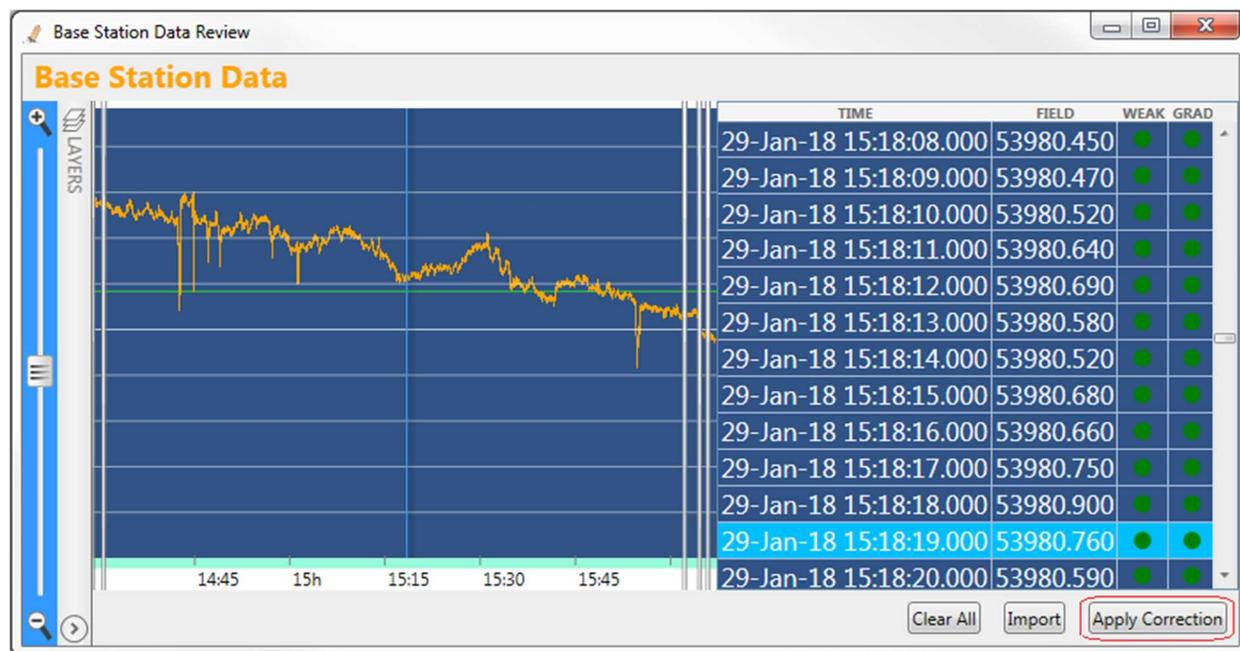
Figure 6-11 - Review and clean up (if necessary) the base station data before applying it to your survey
