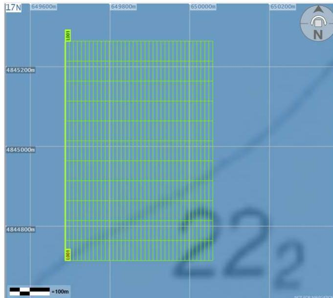
Figure 4-17: Default Guide Grid settings use North-South line orientation with 10m line spacing, and the origin in the NW corner.
