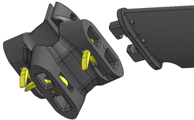
A: Center core with locking levers in the open position
