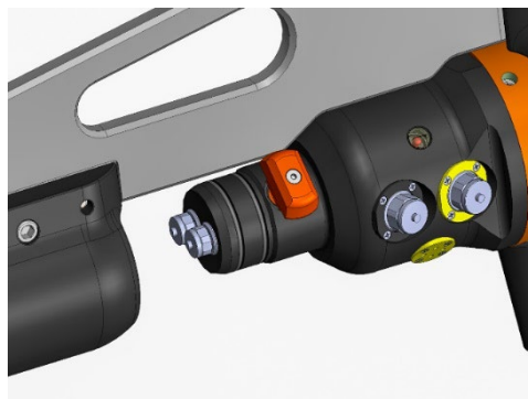
Protective caps on sensor cable connectors on the core module
