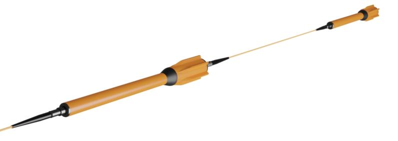
Longitudinal gradiometers offer the largest variation in available baselines, from 1.5m to more than 500m. Long baselines provide superior gradient measurement sensitivity and increased detection ranges. They're also hydro dynamically stable when deployed. Each towfish can be used as a single magnetometer.
