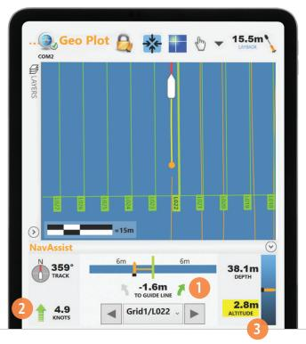
The Geographic Plot shows paths of the GNSS/vessel and the towfish on a coordinate grid, as Latitude/Longitude format or in UTM projection with WGS84 datum. See the precise location of your readings, Markers and Survey Lines.
